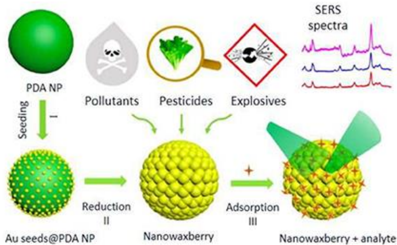
Figure 9. Schematic illustration of the synthesis process of polydopamine @ gold (PDA @ Au) nanowaxberry and its SERS detection. (Reproduced with permission from Chen et al.).
